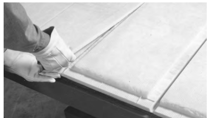
Fig. 2-10. Remove groove scrap. Confirm dimensions. The board is now ready for assembly and closure of a straight duct module, or for fabrication of a fitting.
