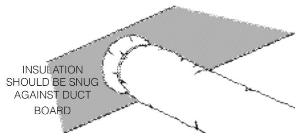
Fig. 4-6E. Install flexible duct to collar according to manufacturer's instructions.
