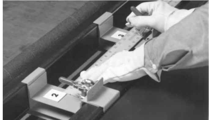
Fig. 2-8. Install tools in grooving machine according to machine manufacturer's instructions, board layout, and cutting plan (see pages 2-10 through 2-13), using either Standard or Preferred tooling set-up (see page 2-10).
