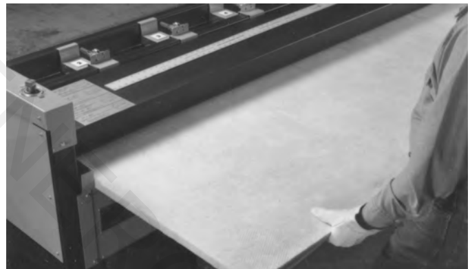
Fig. 2-9. Feed duct board into machine, female shiplap edge first, left hand edge firmly against guide, parallel to rollers. Turn on machine and guide board as friction rollers pick it up and pull it through the cutting tools.
