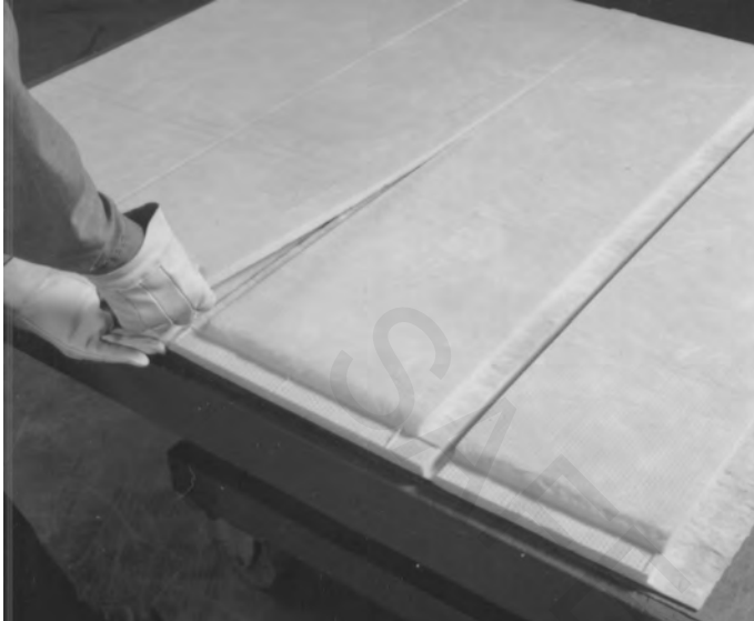
1. Cut shiplaps and corner grooves with hand tools or by machine as shown on pages 2-10 through 2-13. Remove groove scrap. Lifting board as shown will make it easier to remove shiplap groove scrap.
