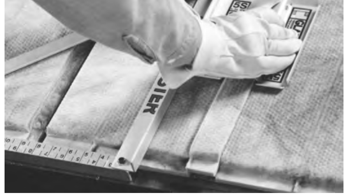
8. Re-position squaring tool to right to make the stapling flap.
