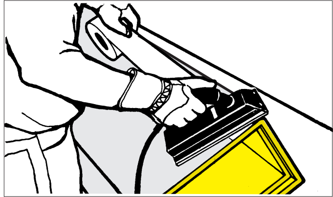
Fig. 4-4A. Apply heat with iron. Do not use a blowtorch; both heat and pressure are required for an effective bond. Complete the bond with a second pass of the iron.
