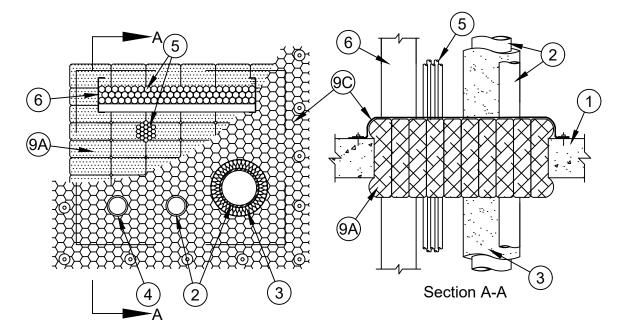
System tested with a pressure differential of 2.5 Pa between the exposed and the unexposed surfaces with the higher pressure on the exposed side.
